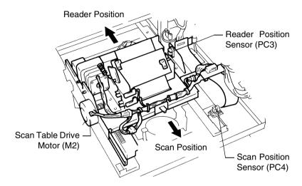
To switch from the Reader Path to the Printer Path, the Scan Table Drive Motor M3 is energized there by moving the Scan Table toward the Printer Position.
